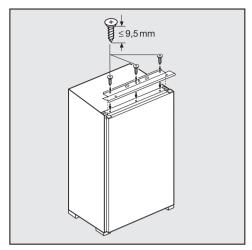
■ Screw the fixing piece to the appliance.
